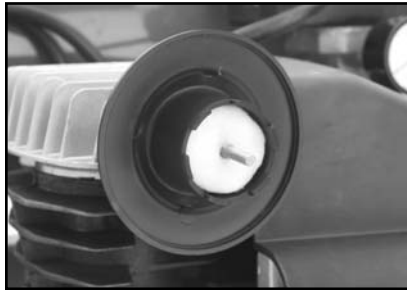
Figure 11. Air filter foam element
